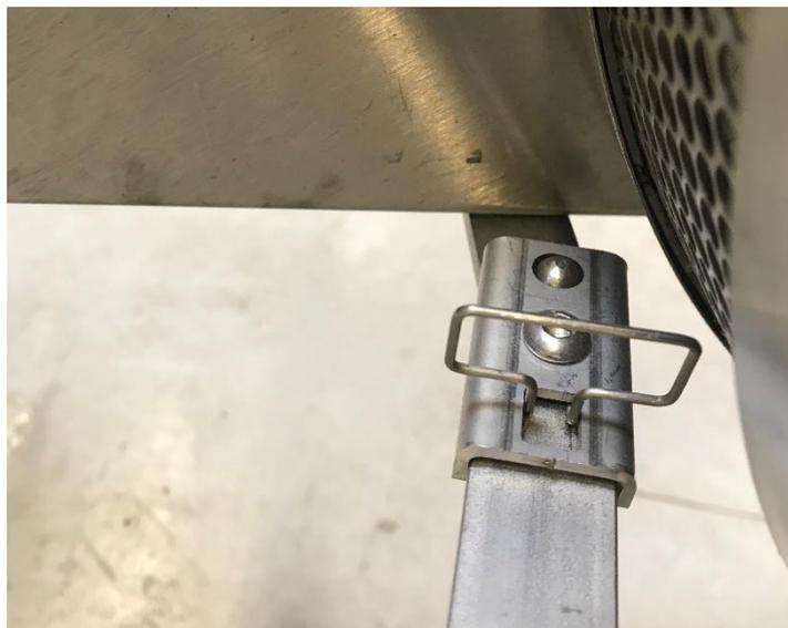
**IMPORTANT:** After connecting the machines together, unlatch them both from their bars and slide them all the way to each end of the bar with no one sat on the machines to ensure they are parallel to avoid damaging your machines when they are used.
